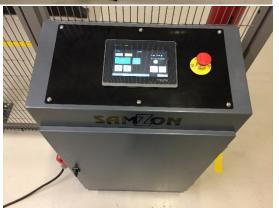
Samzon Pallet-Turner SD is a stationary pallet turner machine that runs to floor-level and is used to change pallets or for removing paper spacer or freezer spacer. The pallet is fed into the machine using a pallet truck or pallet jack. The machine can either rotate 90-degrees or 180-degrees depending on your needs. To remove paper spacer or freezer spacer, the machine is rotated from 0 to 90-degrees, pressure from the platforms is alleviated to allow for removal of spacers.
