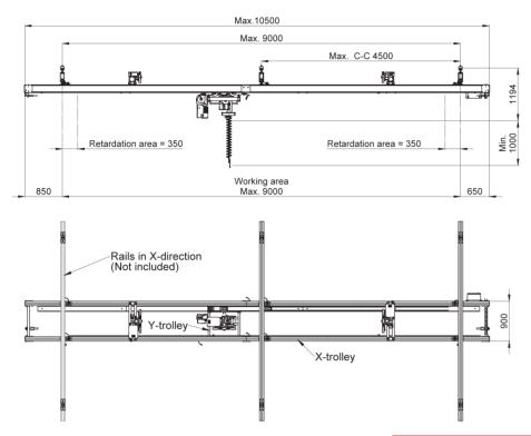
The rail system, Quick-Lift Driven 125i (QLD 125i) is a unique, motorized lifting device that easily covers large areas horizontally, with a lifting load up to 125kg.
