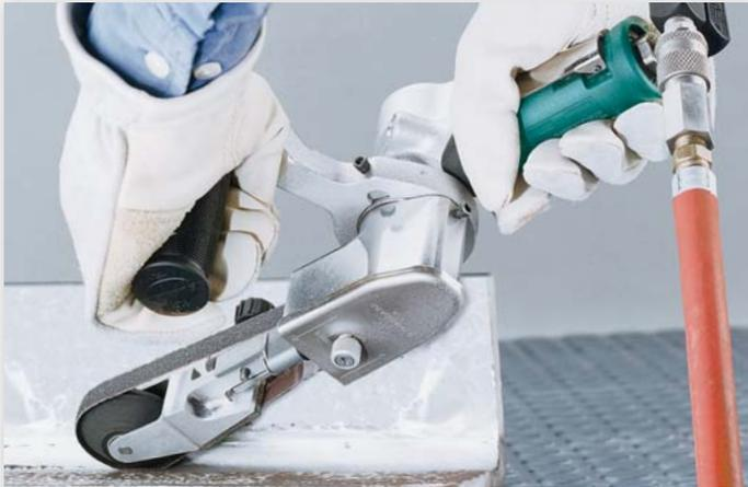
**15300 Dynafiler® III** serves up more power for faster material removal. Corner weld shown is easily taken down with optional **15357 Contact Arm**, with "V" shaped Contact Wheel. This arm is also reversible, effective for both platen sanding and slack polishing.
