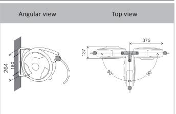
Installation tip for 315 Hose reel Hose reel to be mounted on a wall, pillar or ceiling, minimum 2.5 m above the floor. Hose reel fitted with 2 pcs. screw on firm ground.
