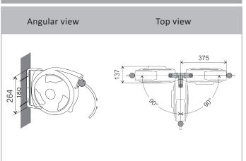
Installation tip for 315 Hose reel Hose reel to be mounted on a wall, pillar or ceiling, minimum 2.5 m above the floor. Hose reel fitted with 2 pcs. screw on firm ground.
