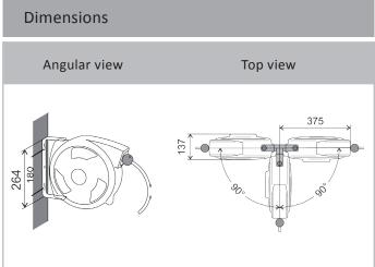
Installation tip for 315 Hose reel Hose reel to be mounted on a wall, pillar or ceiling, minimum 2.5 m above the floor. Hose reel fitted with 2 pcs. screw on firm ground.
