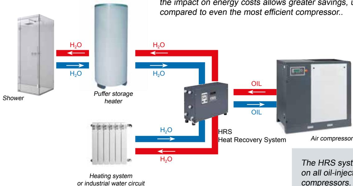
The HRS system can be used on all oil-injected screw compressors.
