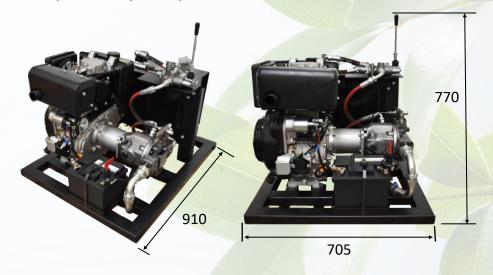
This Hydraulic Power Unit comes with a variable piston pump.
